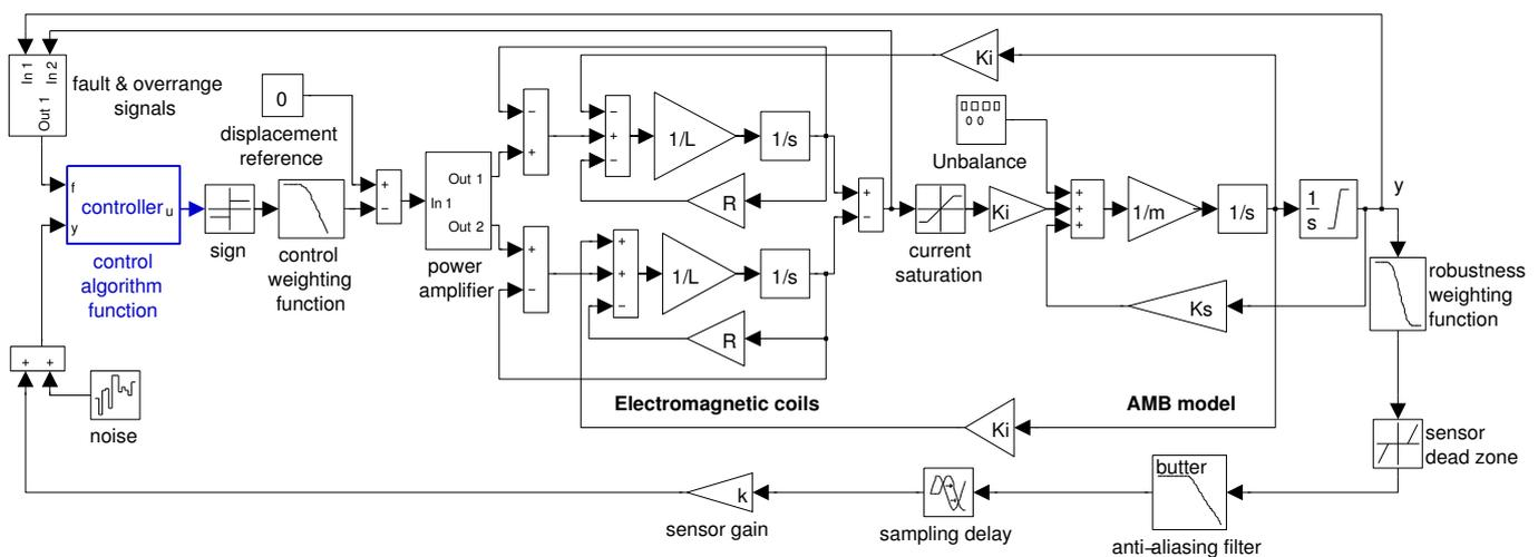
Fig. 1. Single degree of freedom AMB control system
