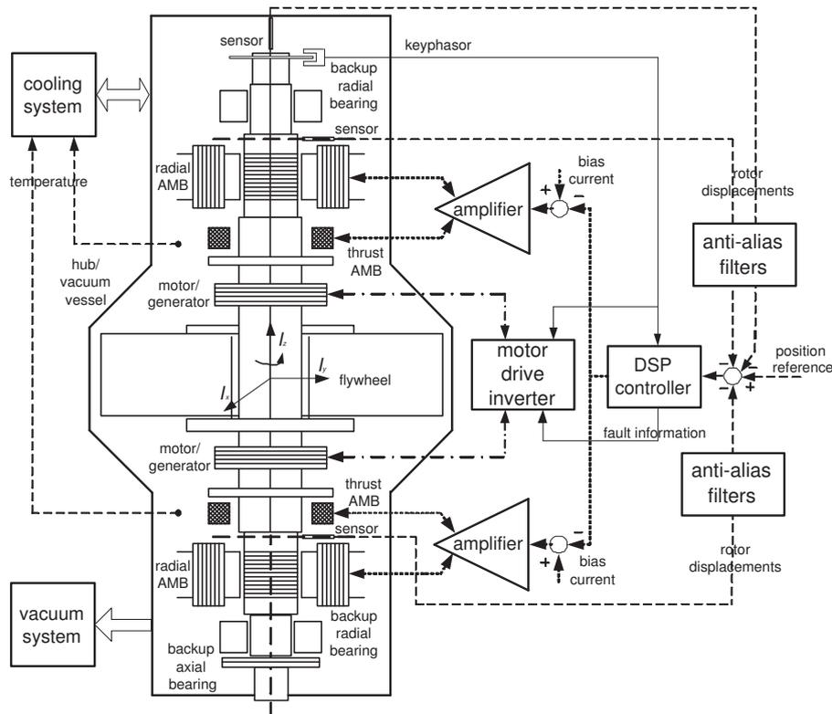
Fig. 3. Flywheel with control, cooling and vacuum system
