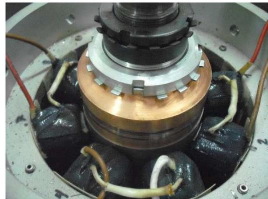
Fig. 2. Heteropolar radial active magnetic bearing
