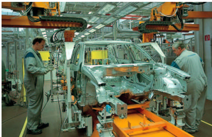
Figure 2. Line Workers using Active Assist Devices to Load Doors onto a Volkswagen Polo frame (Photo courtesy VWVortex)
