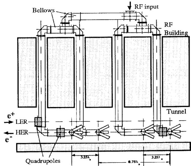
Figure 3. Cross-section of waveguide layout with 4 cavities in tunnel
