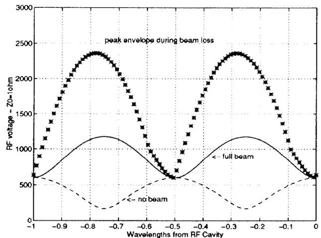
Figure 1. Voltage standing wave pattern in the drive line to a cavity in the low energy ring
