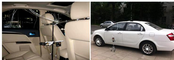
**Fig 3. Photo of the experimental system.**
