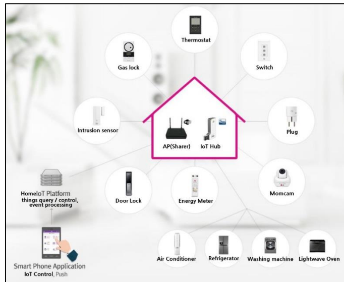
Fig. 1. Figure 1 shows the IoT case of LG telecom. (IoT@home App)
