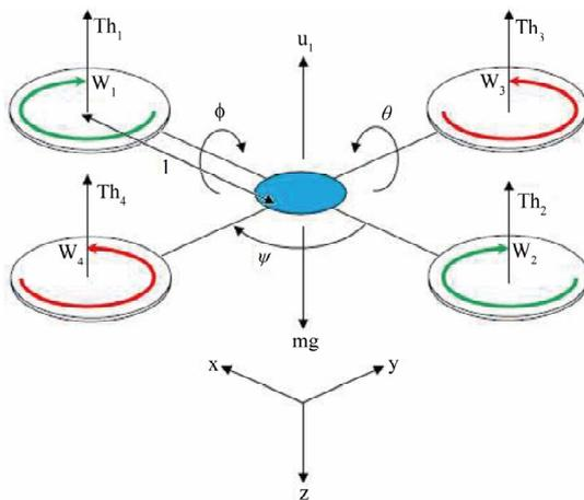
Figure 1. Schematic of Quadcopter.
