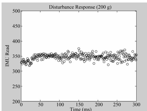
Figure 18. Pitch axis hover test response for 200 g load.
