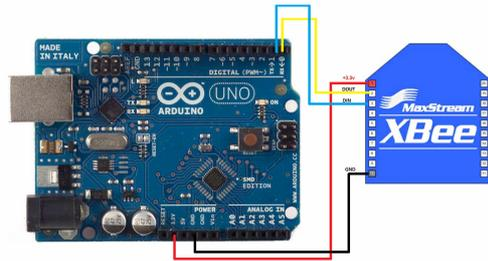
Figure 7. Xbee and Arduino Uno connection.
