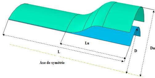
Fig. 2. Dimension of the tube and the die.
