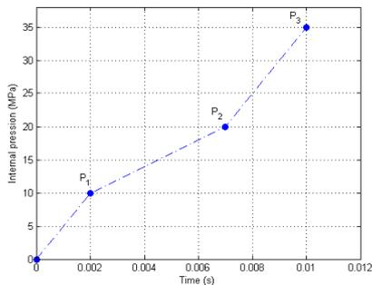
Fig. 4. Load path: pressure (MPa) - time (s).
