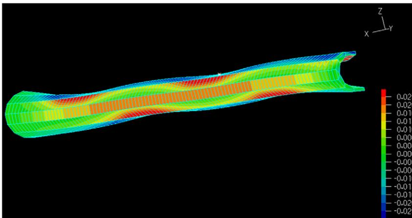
**Figure 10. Microtubule deformation under lateral load.** Deflection is not to scale; the picture illustrates a microtubule half cross-section with half length. Normal strain parallel to the loading plane and orthogonal to the microtubule axis is illustrated in the picture ( $\epsilon_{zz}$ ).
