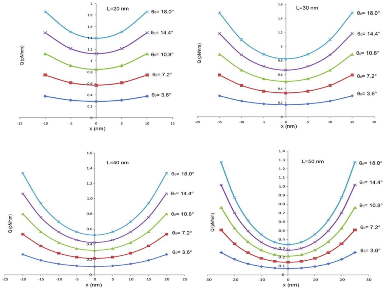
**Figure 9. Microtubule-actin connection load distribution is a function of the angle  $\theta_0$  and the connection length.**
