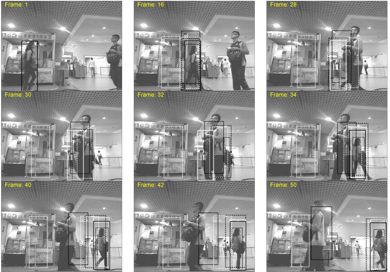
Fig 2. Qualitative Comparison. Color codes: white dashed=A, black dashed=B, white dash-dotted=C, black dash-dotted=D, white solid=E, black solid=F, dark gray solid=Ground truth. (From Left To Right, Top to Bottom) Frame1: All trackers are initialized in the same position, models initiated. –Frame16: Tracker (A) was trapped in background edge clutter. –Frame28: The target is partially occluded, tracker (F) decided to announce the occlusion state to prevent model drift. –Frame30: Full occlusion: all trackers but (F) are updating their models with wrong template i.e. the occluder. –Frame32: End of full occlusion, tracker (E) still searches the same position that loses the target relative to occlude position, tracker (F) still maintains the occlusion state. –Frame34: Recovery from occlusion, tracker (F) with intact models recovers quickly. –Frame40: Tracker (B) lost the main target and start to track occluder due to model drift. –Frame42: Some trackers such as tracker (C) are experiencing fluctuations due to model drifts, yet strong cues such as histogram of depth help them to continue tracking. –Frame50: Trackers lock on the subject again, but tracker (F) does not suffer from model drift and has better tracking performance. (The sequence image is washed out for image clearance. The results are available in color in the first author’s webpage).
