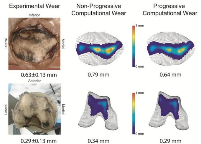
**Figure 2:** Wear results for the patella (top row) and femur (bottom row). Left column is experimental wear areas (white areas are worn regions) and depths. Middle column is predicted wear areas and depths from the non-progressive approach. Right column is predicted wear areas and depths from the progressive approach.
