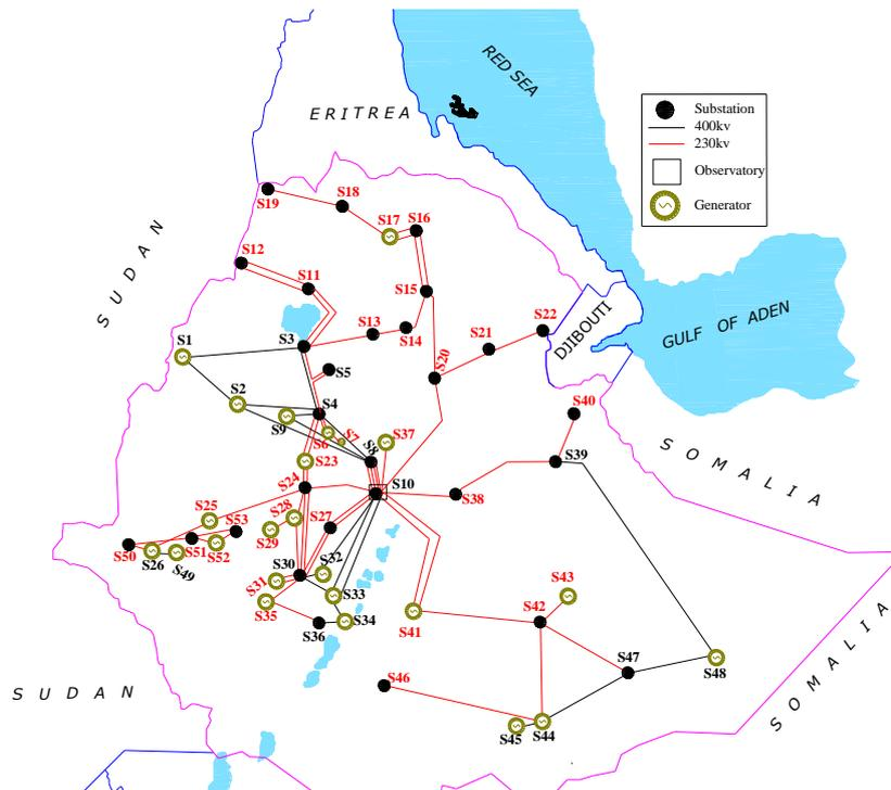
Figure 2. Geographical wiring diagram of dual voltage Ethiopia power grid.
