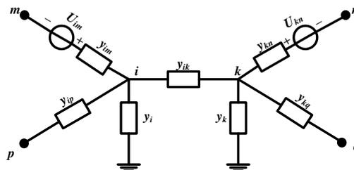
Figure 1. The calculation circuit of GIC node admittance.
