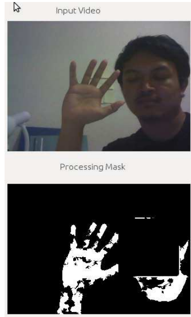
(b) Binary mask obtained using method 3, LCCS
