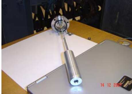
Fig.6 In-vacuum fiber probe for spectroscopic measurements.
