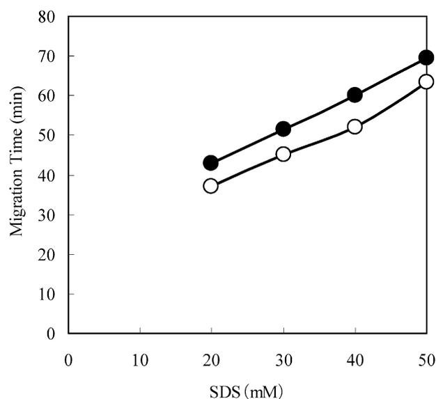
**Fig. 3.** Influence of SDS concentration in the electrophoretic medium on the migration of nobiletin (○) and tangeretin (●). No peak was detected at concentrations of less than 20 mM SDS.
