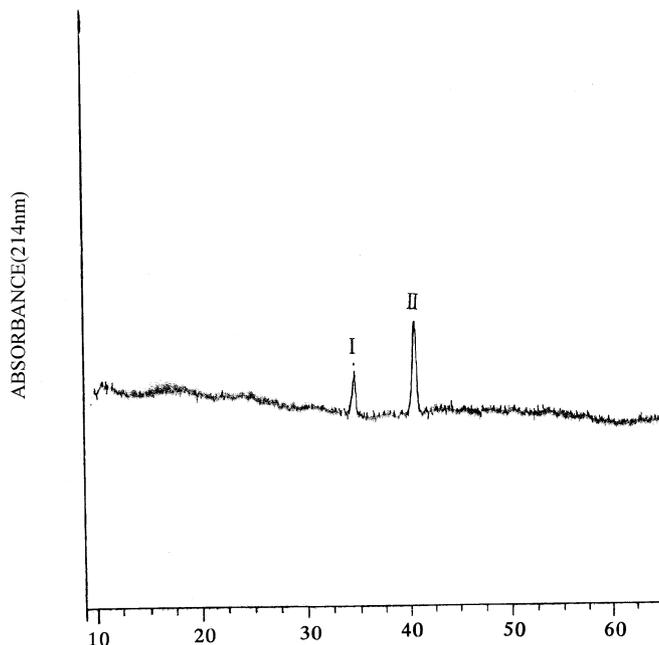
**Fig. 4.** Electrophoretogram of a mixture of nobiletin and tangeretin standards. Conditions: electrophoretic medium, pH 7.0 buffer solution (32mM SDS-20mM NaH<sub>2</sub>PO<sub>4</sub>-12mM Na<sub>2</sub>B<sub>4</sub>O<sub>7</sub>-20% MeOH); voltage, 21 kV; capillary, 54.5 cm (detection point), 60 cm (Total length)×75μm I.D.; untreated fused-silica capillary. Peak: I =nobiletin (0.25 mg/mL); II=tangeretin (0.25 mg/mL).
