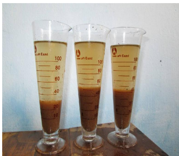
Fig. 5 Volume of biofloc was determined by Imhoff glass [14].
