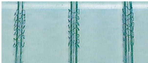
**Figure 1.** Magnified portion of phantom stage 3. Phantoms were 4.0-mm Wiktor stents with “restenotic” lumen diameter of 2.0, 2.5, and 3.0 mm.
