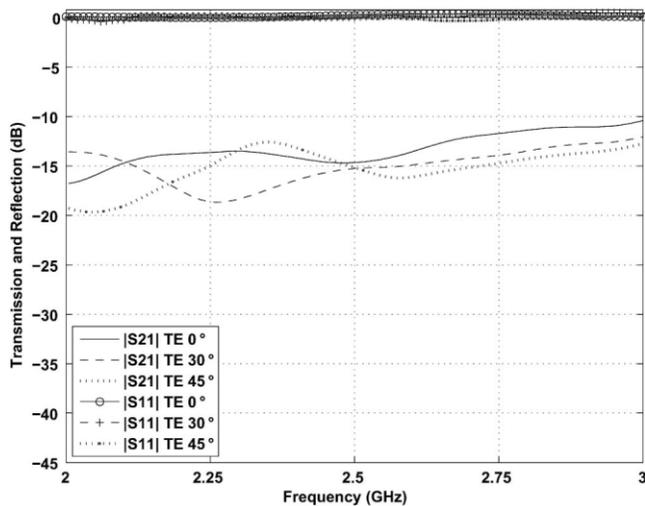
**Figure 4** Measured transmission and reflection characteristics of the single-layer active FSS when the diodes are in ON state
