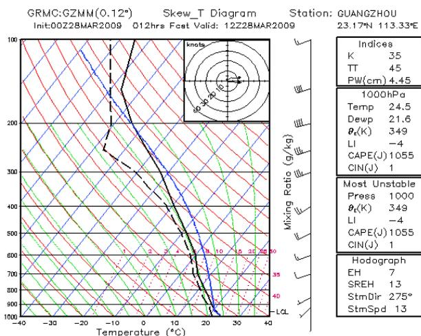
**Fig. 4.** Atmospheric sounding in Guangzhou ( $113.33^{\circ}\text{E}$ ,  $23.17^{\circ}\text{N}$ ) at 00:00 UTC on 28 March 2009. The black solid line corresponds to the temperature, and the black dash line represents the dew point temperature.
