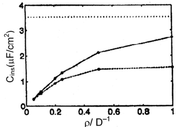
Fig. 2—Insulator capacitance  $C_{ins}$  versus the tube density  $\rho$  (normalized to  $\rho_{max}=1/D$ , the close-packed case) for an array of parallel nanotubes, compared to  $C_{ins} = K_{ins} \epsilon_0/t_{ins}$  of the MOS capacitor (dotted line). The solid line assumes classical charge distribution and dash line one sub-band quantum limit.
