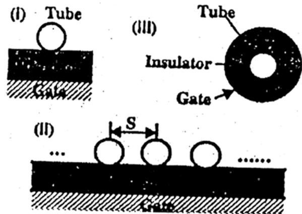
Fig. 1—Three geometries of nanotube MIS capacitors: (i) the nanotube planar capacitor, (ii) a periodic array of nanotubes, and (iii) the coaxially gated capacitor; nanotube diameter  $D=1$  nm,  $t_{\text{ins}}=1$  nm, and  $\kappa_{\text{ins}}=4$  are the same for all capacitors[9]
