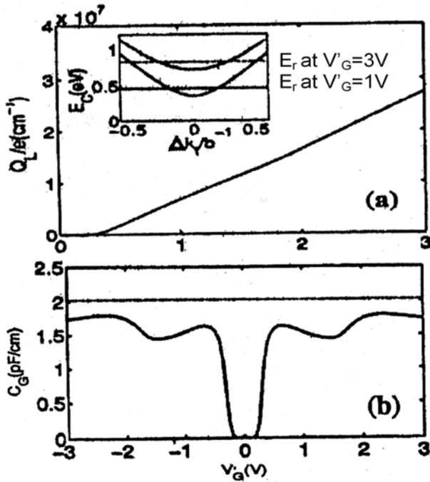
Fig. 3—Charge versus gate voltage for the co-axial capacitor, (a) charge density  $Q_L$  and (b) the gate capacitance  $C_G$  Vs. the effective gate voltage  $V_G^-$ . The inset in (a) shows location of the fermi level in the first and second sub-bands as  $V_G^-=1V$ , and  $3V$ . The dotted line in (b) indicates the insulator the capacitance  $C_{ins}$  (Ref. 9).
