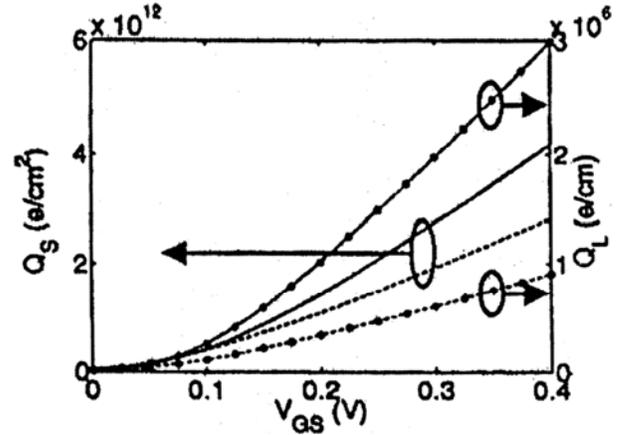
Fig. 4—Charge density versus gate voltage  $v_G$  on the left axis, the close packed array of nanotubes (dash line) is compared to the Si MOS capacitor (solid line). On the right axis, the co-axially gated capacitor (solid with circles) is compared to the single nanotube planar geometry (dashed with circles). To make a fair comparison, the gate were function of each capacitor is adjusted to produce a common threshold voltage,  $V_T \approx 0.1V$  (Ref. 9).
