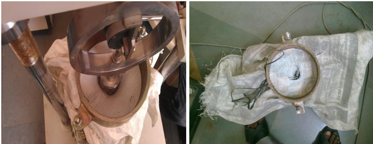
Photo: CBR Plunger Push through Test (ASTM D4833). Before and after rupture of the specimen.
