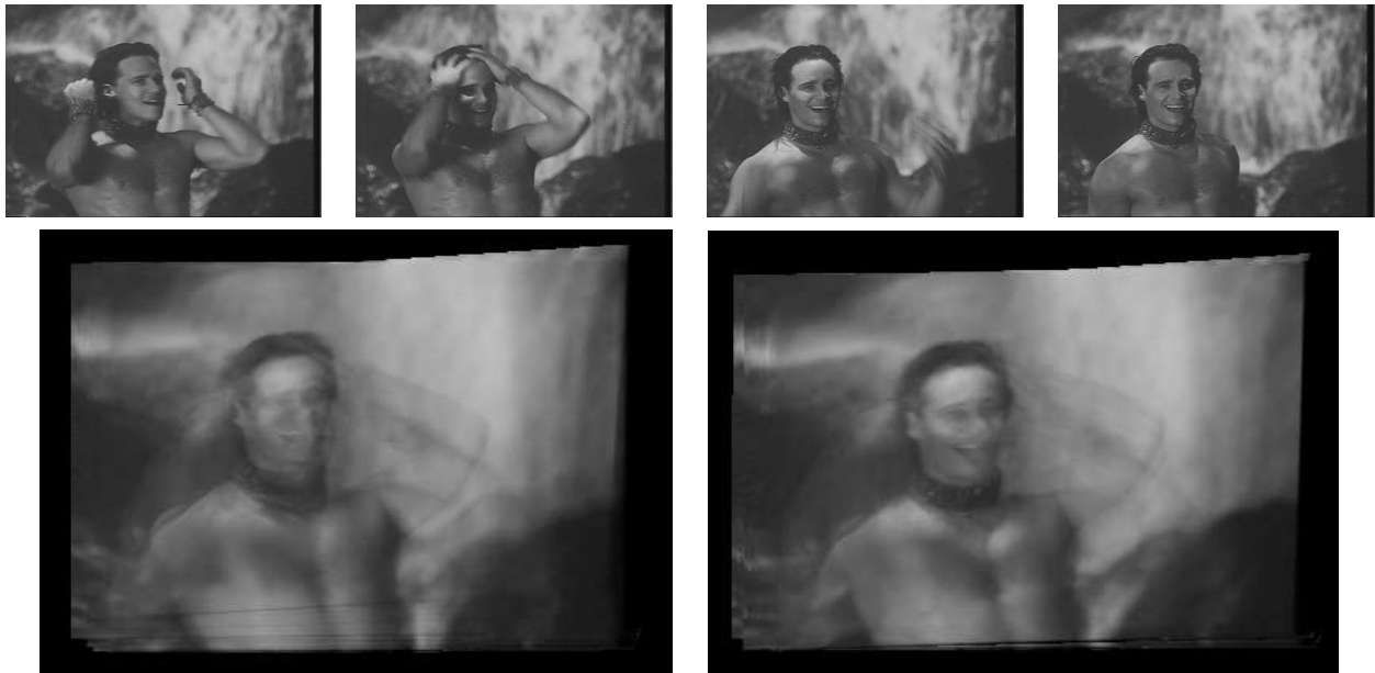
Figure 6. Four frames from a sequence containing several motions and high dominance ambiguity (top) and layers obtained with temporally localized (bottom-left) and with the spatiotemporal model (bottom-right). The spatiotemporal model leads to better image registration, and perceptually more meaningful content-summation.
