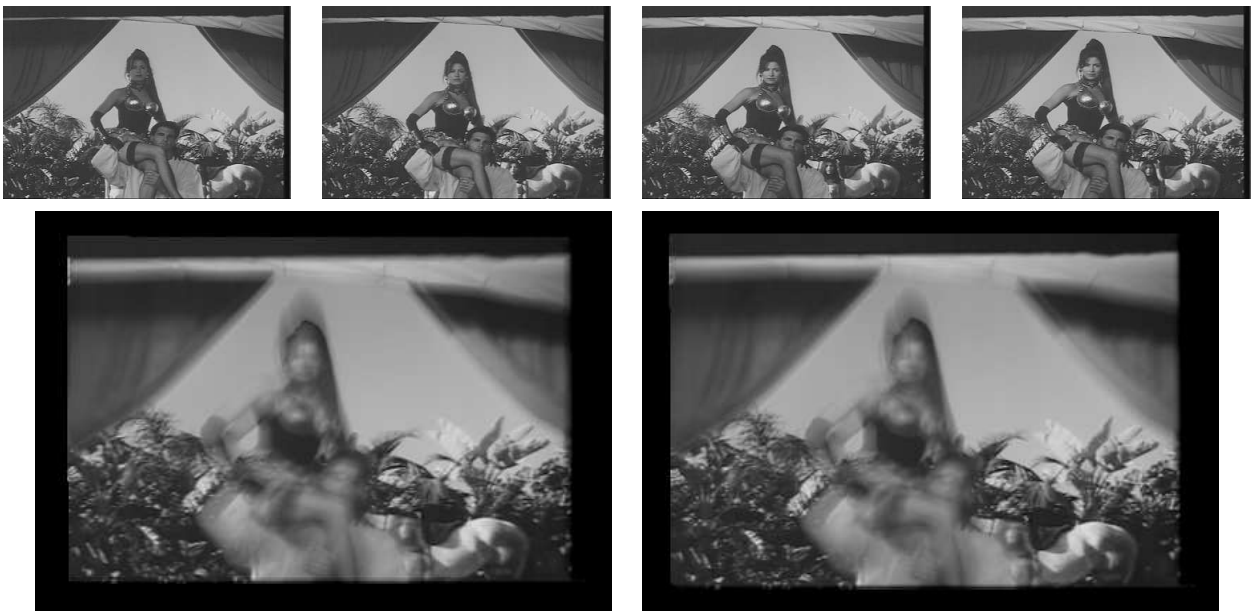
Figure 5. Four frames from a sequence containing two motions but reduced dominance ambiguity (top) and layers obtained with temporally localized (bottom-left) and with the spatiotemporal model (bottom-right). The layers are identical.
