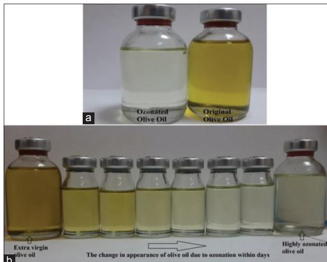
**Figure 2:** Together with ozonation, the olive oil begins to lose its original color. This situation shows the saturation with oxygen of double bounds in unsaturated fatty acids. Highly ozonated oil is more transparent and viscous than olive oil
