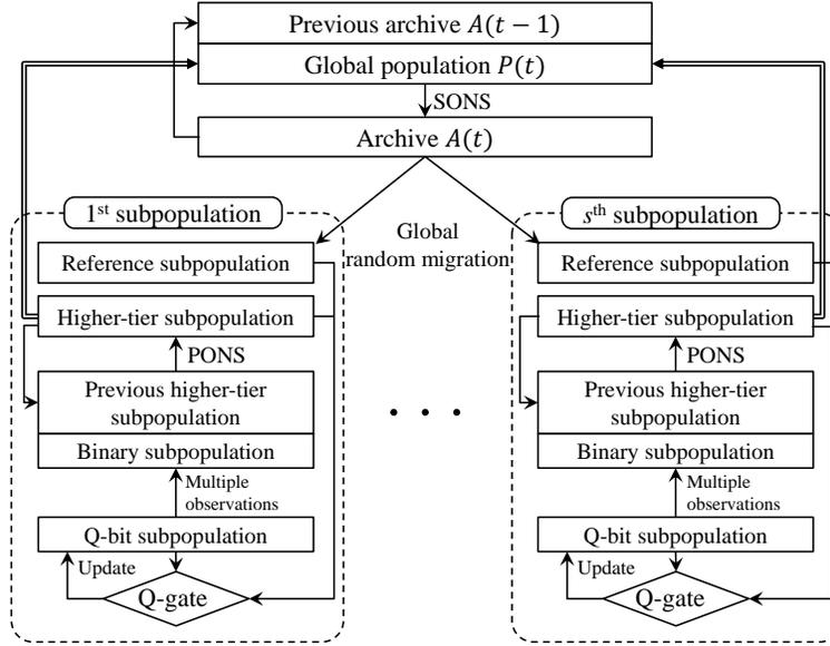
Fig. 2: Overall procedure of DMQEA, where PONS: Primary objectives-based nondominated sorting, SONS: Secondary objectives-based nondominated sorting
