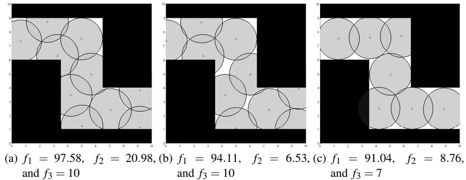
Fig. 3: The optimized sensor arrangements considering mostly (a) sensor coverage (b) interference rate (c) the number of sensors
