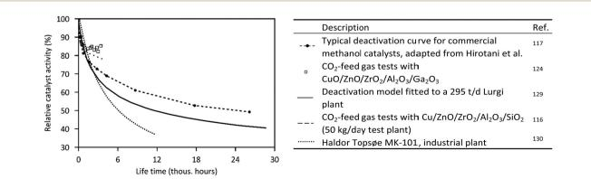
Fig. 5 Deactivation curves of commercial methanol catalysts.<sup>116,117,124,129,130</sup>
