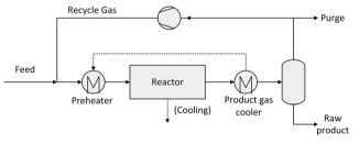
Fig. 3 Conventional synthesis loop in methanol, DME and FT-processes.
