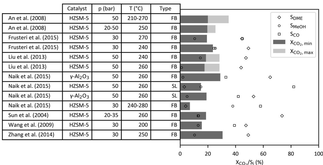
Fig. 18 Overview of CO<sub>2</sub> conversion and selectivity of DME, methanol and CO ( $S_i = i/[CO_{2,in} - CO_{2,out}]$ , with  $i = 2 \times$  DME/MeOH/CO, based on amount of C-atoms) of direct hydrogenation experiments of CO<sub>2</sub> to DME.<sup>306,310,313,314,317–319</sup>
