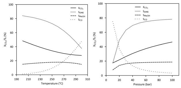
Fig. 13 Equilibrium conversion of CO<sub>2</sub> (=  $[CO_{2,in} - CO_{2,out}]/CO_{2,in}$ ) and selectivity of DME, methanol and CO ( $S_i = i/[CO_{2,in} - CO_{2,out}]$ , with  $i = 2 \times DME/MeOH/CO$ , based on amount of C-atoms) dependent on (a) temperature and (b) pressure ( $H_2: CO_2 = 3: 1$ , based on Aspen Plus Simulation).
