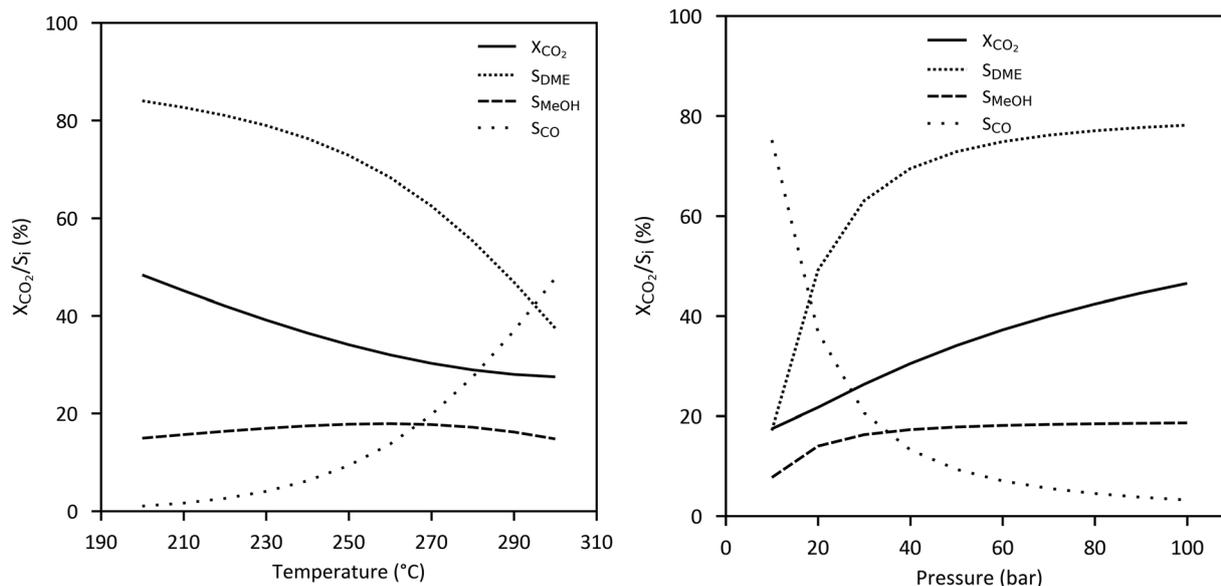
Fig. 13 Equilibrium conversion of CO<sub>2</sub> ( $= [\text{CO}_{2,\text{in}} - \text{CO}_{2,\text{out}}]/\text{CO}_{2,\text{in}}$ ) and selectivity of DME, methanol and CO ( $S_i = i/[\text{CO}_{2,\text{in}} - \text{CO}_{2,\text{out}}]$ , with  $i = 2 \times \text{DME/MeOH/CO}$ , based on amount of C-atoms) dependent on (a) temperature and (b) pressure ( $\text{H}_2 : \text{CO}_2 = 3 : 1$ , based on Aspen Plus Simulation).
