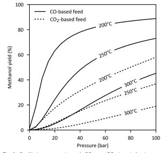
Fig. 4 Equilibrium conversion of CO- or  $\rm CO_2$ -based feed gas to methanol.
