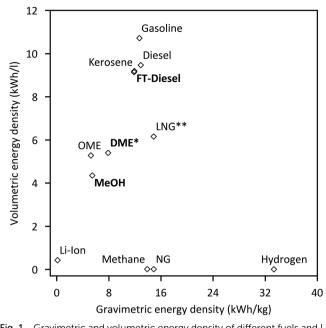
Fig. 1 Gravimetric and volumetric energy density of different fuels and Lilon batteries for comparison (\*at 10 bar; \*\*at -160 °C).<sup>13-15</sup>
