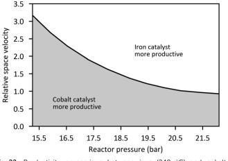
Fig. 22 Productivity comparison between iron (240  $^\circ\text{C})$  and cobalt (220  $^\circ\text{C})$  based catalysts. Adapted from Steynberg and Dry.  $^{35}$
