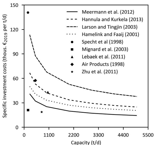
Fig. 10 Specific investment cost curves of methanol synthesis loop including purification normalized to the year 2019.<sup>228,232,239–245</sup>
