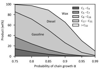
**Fig. 21** Fischer–Tropsch product distribution as a function of the chain growth probability, calculated on a mass fraction basis. The number of carbon atoms per chain is shown.
