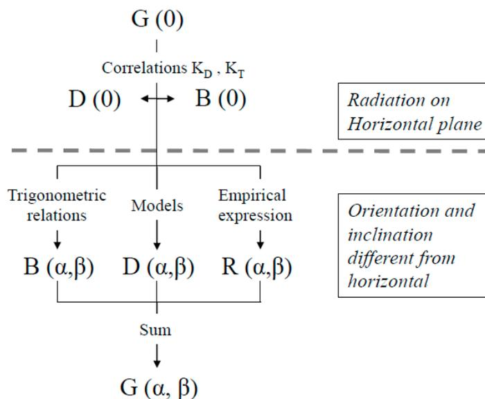
**Figure 1.** Diagram for the calculation of the global solar radiation on a non-horizontal surface (orientation (α) and inclination (β)).
