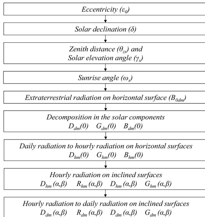
**Figure 2.** General calculation procedure for obtaining solar radiation at any inclination and orientation.
