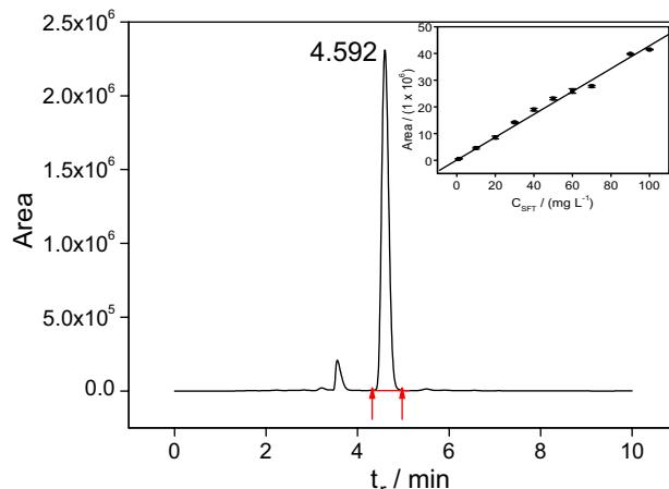
**Figure 6.** Analytical curve obtained by HPLC in the presence of soil. Parameters: mobile phase containing H<sub>2</sub>O/ACN 50:50 (v/v); mobile rate: 1.0 mL min<sup>-1</sup>; injection volume: 20 µL; column temperature: 30 °C; wavelength: 214 nm and Shimadzu C<sub>18</sub> column.
