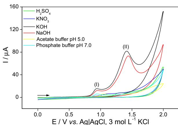
**Figure 2.** Cyclic voltammograms obtained with the GCE using 0.10 mol L<sup>-1</sup> solutions of: KOH; NaOH; KNO<sub>3</sub>; phosphate buffer pH 7.0; acetate buffer pH 5.0 and H<sub>2</sub>SO<sub>4</sub> as the supporting electrolyte solution in the analysis of 1.00 mmol L<sup>-1</sup> of sulfentrazone.
