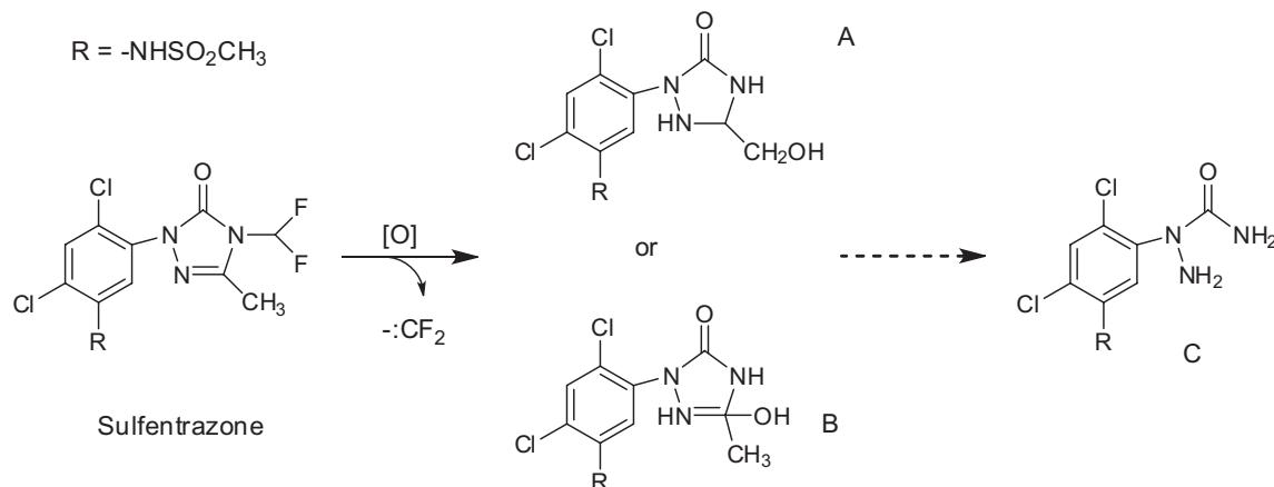
**Scheme 1.** A possible route for the electrochemical oxidation of sulfentrazone.
