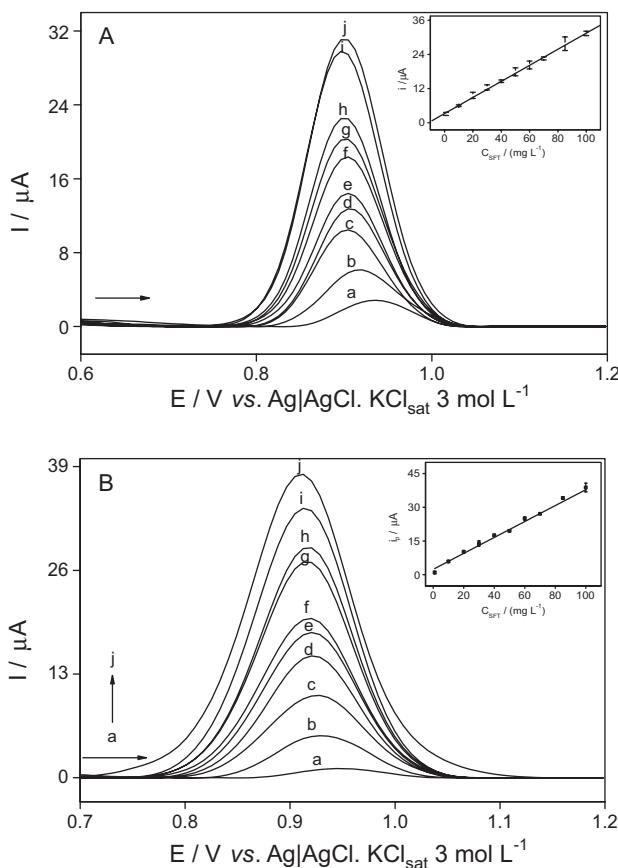
**Figure 5.** Analytical curves in the absence of soil (A) DPV electrooxidation of sulfentrazone at different concentrations: blank; (a) 5.0; (b) 10.0; (c) 20.0; (d) 30.0; (e) 40.0; (f) 50.0; (g) 60.0; (h) 70.0; (i) 85.0 and (j) 100.0 mg L<sup>-1</sup> and in presence of soil; (B) DPV electrooxidation of sulfentrazone at different concentrations: as stated above. Conditions: GCE in 0.10 mol L<sup>-1</sup> KOH as supporting electrolyte solution.
