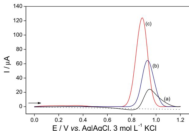
**Figure 3.** Comparison between (a) LSV; (b) SWV and (c) DPV experiments in optimized conditions for  $1.00 \text{ mmol L}^{-1}$  SFT at GCE in  $0.10 \text{ mol L}^{-1}$  KOH.
