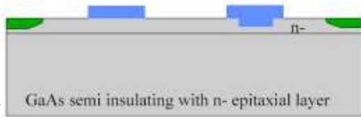
Etch Away Remaining Oxide
