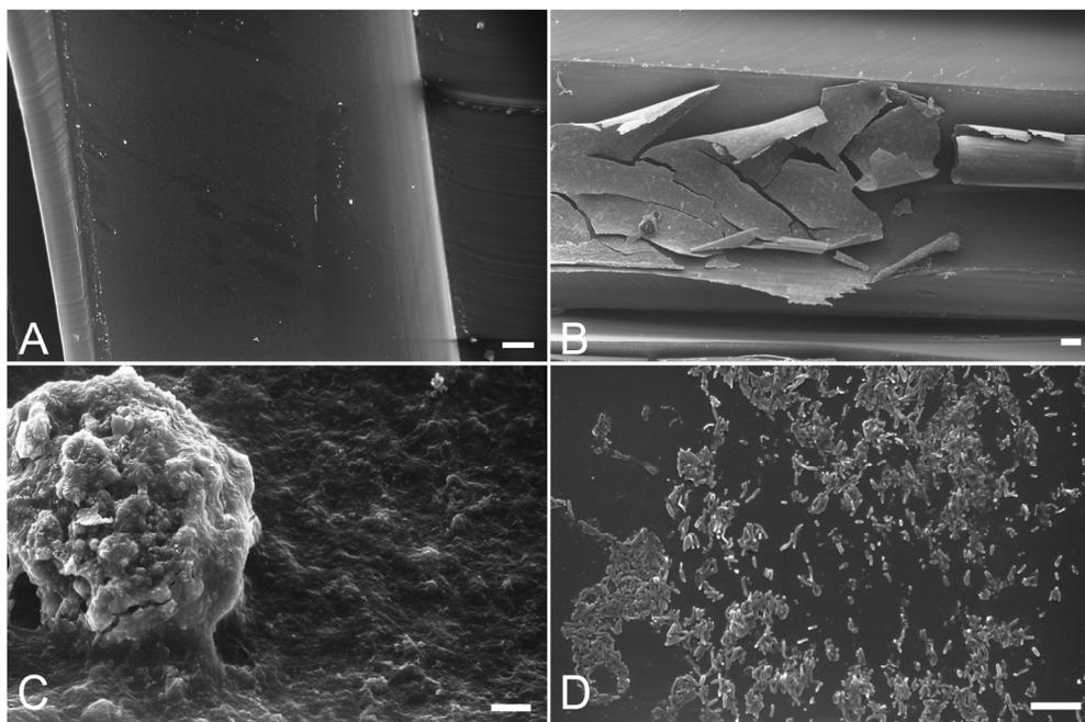
Notes: (A) Control sample of an unused tube. Scale bar = 100μm; (B) Loosely adherent biofilm detached from the tube surface. Scale bar = 100 μm; (C) Bulk, bulging material. Scale bar = 10μm; (D) Clusters of rod-shaped bacteria. Scale bar = 10μm.
