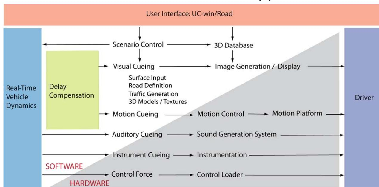
**Figure 3:** Software and Hardware system components [3]
