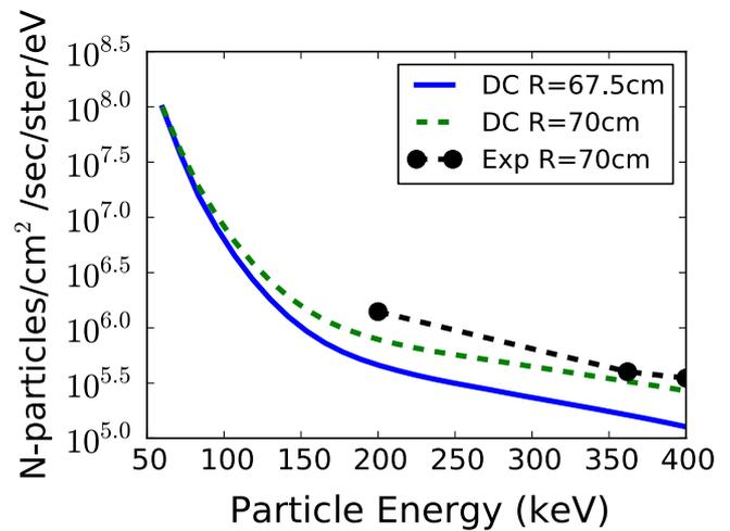
**Figure 8.** CNPA energy spectra from CQL3D using DC Lorentz orbit based coefficients at  $t = 4$  ms. Two vertical view chords at  $R = 70$  cm and 67.5 cm at the midplane calculated from CQL3D/DC are compared to the experimental measurement at 0–10 ms for  $R = 70$  cm from figure 7. The DC coefficient case for  $R = 70$  cm shows excellent agreement with the experimental measurement.
