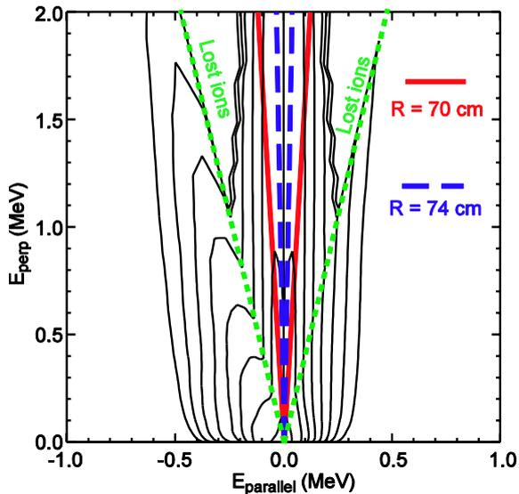
**Figure 2.** The distribution function resulting from self-consistent coupling between AORSA and CQL3D for a minority heating case shown at a normalized minor radius of  $r/a = 0.3$ . The green dashed lines indicate the region in momentum space where ions become trapped. The solid red and dash blue lines show which trapped ions are viewed by the compact neutral particle analyzer (CNPA) ion diagnostic discussed in section 4.2.
