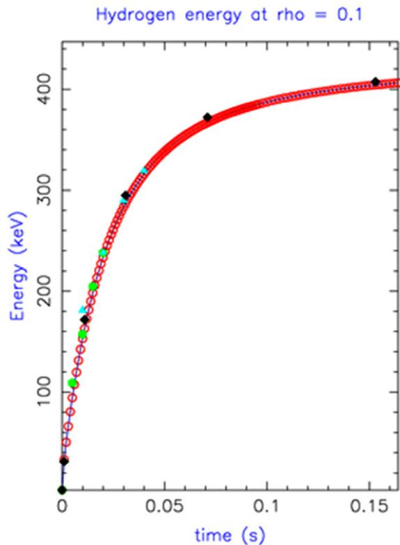
**Figure 5.** Implicit versus explicit time advance for evolution of minority ion distribution using CQL3D-AORSA codes. The maximum energy on the mesh was 2000 keV. The toroidal mode was  $n_\phi = 10$  and the RF power was 2.65 MW. Hollow (red) circles are explicit steps and filled (black) diamonds show using 5 stationary points in each MPE cycle. Filled (green) circles show using four stationary points in each MPE cycle.
