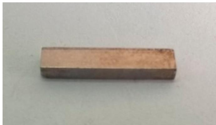
**Figure 1.** Sample of magnetic controlled shape memory alloy (MSMA) for the experiment.
