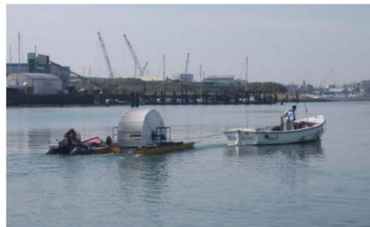
Figure 15 Experimental setup for the towed tests of the demonstrator tidal mill
