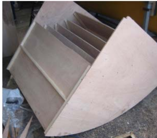
Figure 10 Completed construction of one quarter of the waterwheel.
