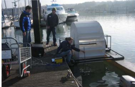
Figure 14 Experimental setup for the tests of the demonstrator tidal mill using the engine to accelerate the flow
