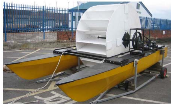
Figure 13 The completed tidal mill with the waterwheel in place.
