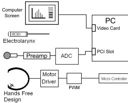
Figure 5: Block diagram of test set up.
