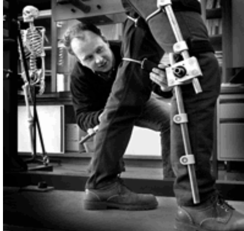
Figure 1.1: The exoskeleton, consisting of the frame, the hip and the knee
