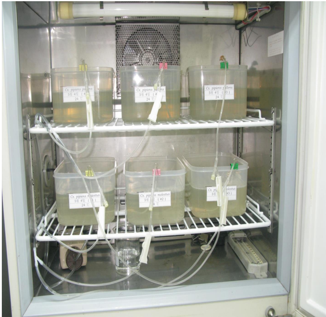
Fig1 The arrangement of egg-hatching containers in the growth chamber for development under controlled temperature with aeration system shown
