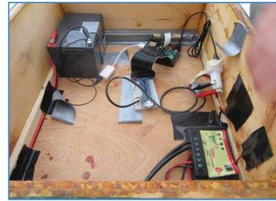
Figure 1. BeePi hardware components
