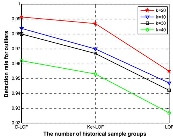
**Figure 3.** Detection rate for outliers with different  $k$  values.
