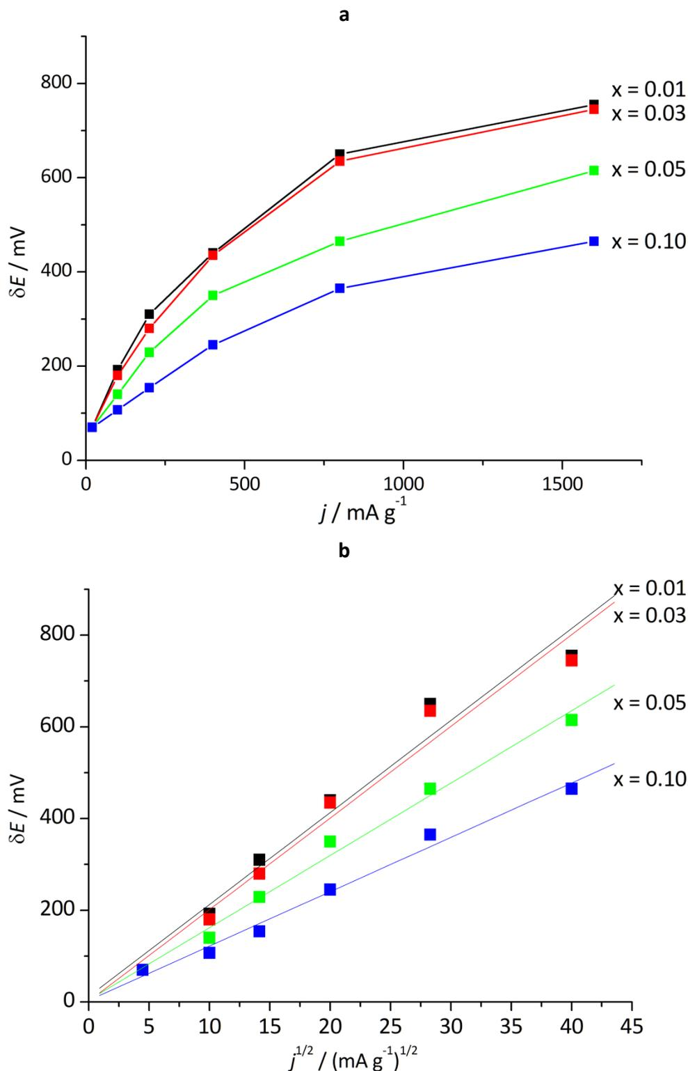
**Figure 4.** **a** - Electrode polarization vs. current density for doped LFP; **b** - Electrode polarization vs. square root of current density for doped LFP. The straight lines are drawn by minimal squares method
