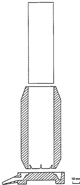
FIGURE 3 Cross-section of the stainless steel tool used in the hydraulic leaf press
