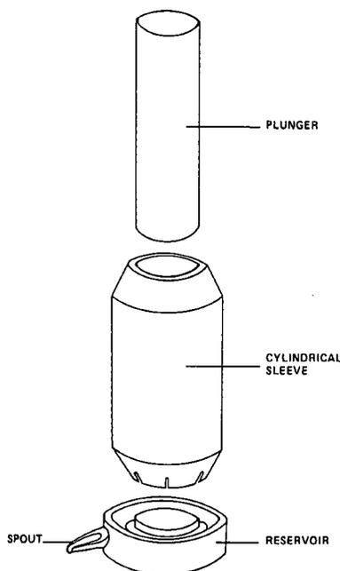
FIGURE 4 Isometric drawing of plunger, sleeve and reservoir
