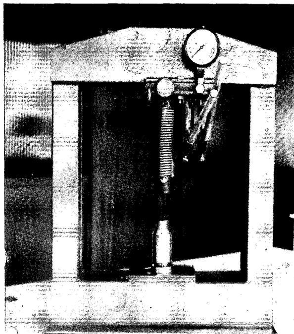
FIGURE 1 Hydraulic ram press for extracting fluids from leaf tissue
