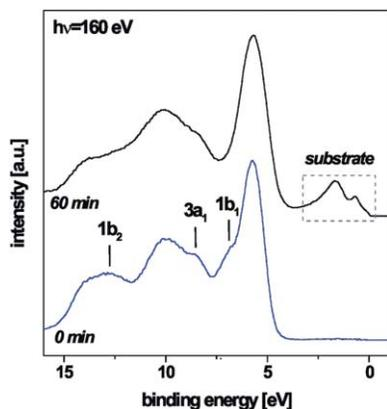
FIG. 5. Valence band photoemission spectra obtained from the as-grown G6W10 and from the same film after 60 min of x-ray irradiation.
