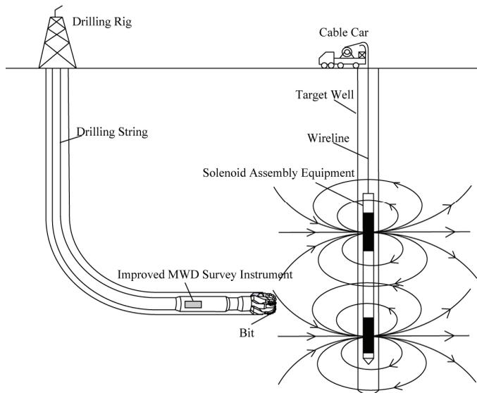
Figure 1: A Schematic diagram of the principle of SARS for a down-hole intersection of two wells
