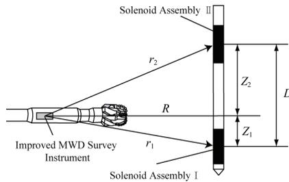
Figure 5: Side view of geometrical relationship between the solenoid assembly equipment and the MWD survey instrument
