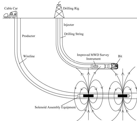
Figure 6: Schematic diagram of SARS working for twin horizontal SAGD wells
