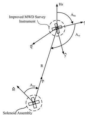
Figure 7: Axonometric view of the geometrical relationship between the improved MWD survey instrument and the solenoid assembly equipment
