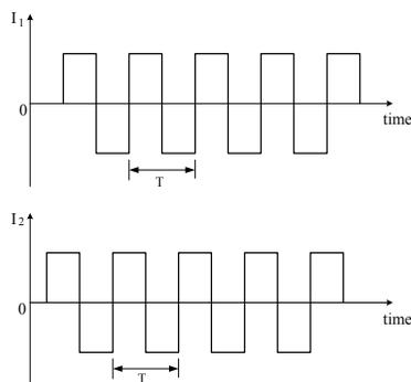
Figure 3: Currents in two orthogonal column-solenoids in each solenoid assembly
