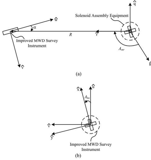
Figure 4: Geometrical relationship between the solenoid assembly equipment and the improved MWD survey instrument
