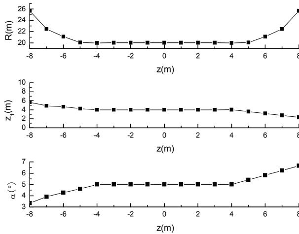
Figure 9: The variation of the calculating  $R$ ,  $z_1$ , and  $\alpha$  versus  $z$ .
