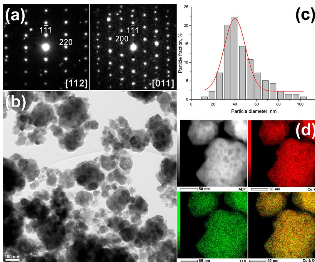
**Figure 2.** Characterization of  $\text{Co}_3\text{O}_4$  nanoparticles by TEM: (a) typical ED patterns of the  $\text{Co}_3\text{O}_4$  along main crystallographic zone axes  $[\bar{1}12]$  and  $[011]$ ; (b) bright field low magnification TEM image; (c) particle size distribution calculated from TEM images; (d) energy-dispersive X-ray spectroscopy (EDX) elemental maps of Co (red), O (green) and their mixture.
