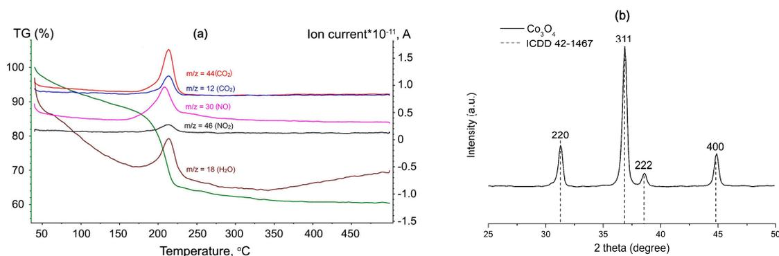
**Figure 1.** (a) TG-MS curves for of the dried precipitate; (b) X-ray diffraction patterns of  $\text{Co}_3\text{O}_4$  nanoparticles.
