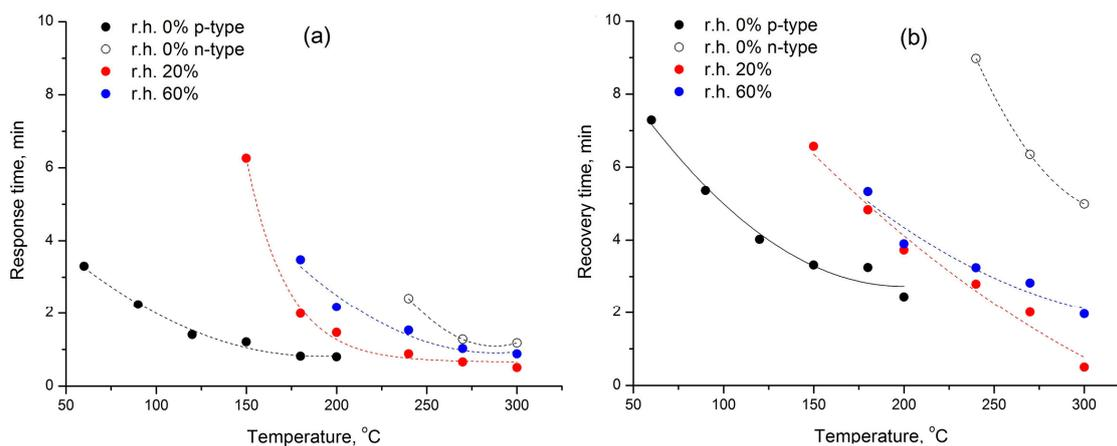
**Figure 12.** Values of response (a) and recovery (b) time as a function of temperature at 0, 20 and 60% r.h.
