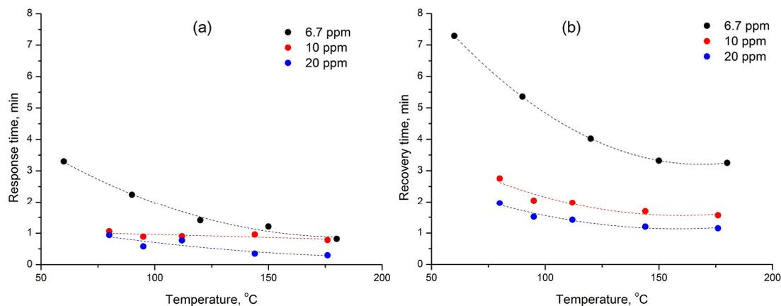
**Figure 11.** Values of response (a) and recovery (b) time as a function of temperature at 0% r.h.
