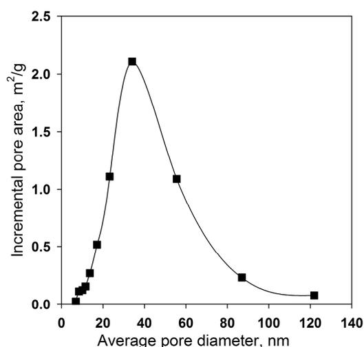
**Figure 4.** Pore size distribution calculated by BJH method.
