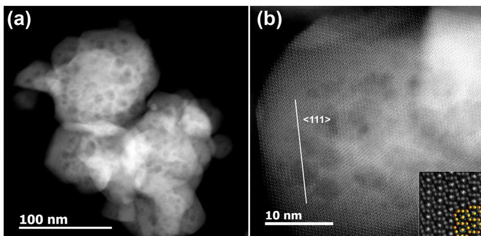
**Figure 3.** (a) Low-magnification and (b) high resolution HAADF-STEM images of  $\text{Co}_3\text{O}_4$  nanoparticles viewing along the [011] zone axis. An enlarged image with overlapped structural model (Co—orange, O—blue) is given as inset.
