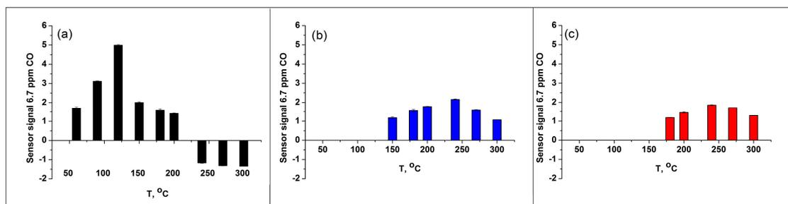
**Figure 9.** Bar chart showing the 6.7 ppm CO response of the  $\text{Co}_3\text{O}_4$  sensor as a function of temperature at 0% r.h. (a), 20% r.h. (b), and 60% r.h. (c). The area of “negative” values in the temperature range 240–300 °C in dry air (part (a)) corresponds to n-type sensor behavior.
