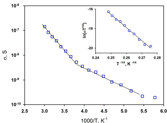
Figure 6. Temperature dependence of the conductivity of nanocrystalline  $\text{Co}_3\text{O}_4$  thick film. Inset: temperature dependence of the conductivity in the Mott VRH model coordinates.
