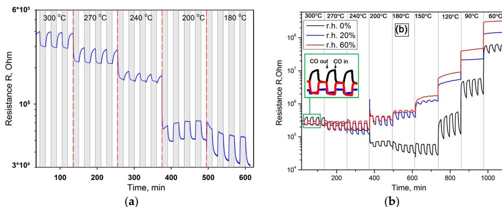
**Figure 8.** (a) Electrical response of  $\text{Co}_3\text{O}_4$  to the periodic change of gas phase composition from 6.7 ppm CO/air (15 min) to pure air (15 min) (0% r.h.) in dry (a) and humid (b) conditions. On part (a) the time periods when CO is introduced into sensor chamber are marked by gray color.
