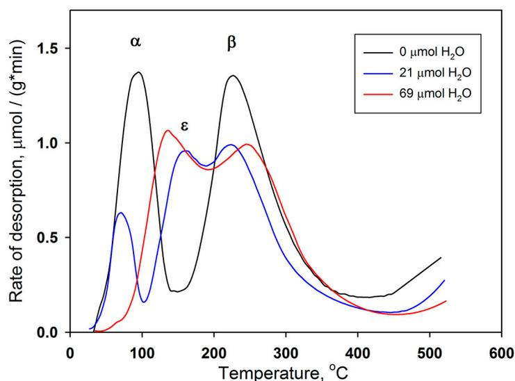
**Figure 10.** TPD curves of oxygen obtained after procedures consisting in oxygen adsorption after pre-adsorption of different quantity of water (0, 21 or 69  $\mu\text{mol/g Co}_3\text{O}_4$ ). Adapted from [34].
