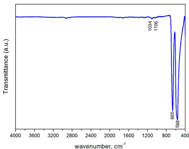
Figure 5. FT-IR spectra of  $\text{Co}_3\text{O}_4$  nanoparticles.
