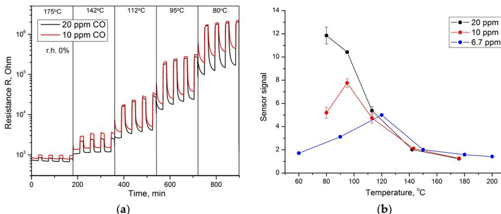
**Figure 7.** (a) Electrical response of  $\text{Co}_3\text{O}_4$  to the periodic change of gas phase composition from dry air (30 min) to CO/air (15 min); (b) sensor response of the  $\text{Co}_3\text{O}_4$  to CO (0% r.h.) as a function of temperature.
