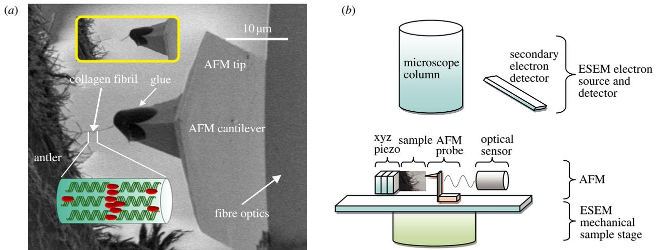
Figure 1. (a) SEM image showing a typical testing configuration. A large number of exposed CFs observed at the fracture surface of antler bone. An individual CF protruding from the fracture surface is attached to the glue at the end of the AFM probe. Translation of the AFM probe away from the fibril causes tensile deformation of the fibril until failure occurs, which is shown in the inset image. (b) Schematic showing set-up of combined SEM–AFM. (Online version in colour.)
