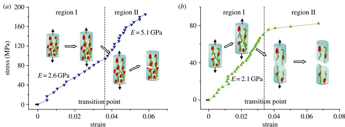
Figure 5. Tensile stress–strain curves for MCFs showing two distinct mechanical behaviours. Tropocollagen uncoiling occurs initially in both types of fibrils within region I. In (a), the fibril shows an enhanced elastic modulus in region II owing to mineral increasing the stress transfer between tropocollagen macromolecules. In (b), the low mineral density within the fibrils allows sliding between tropocollagen molecules, resulting in a plastic deformation. (Online version in colour.)
