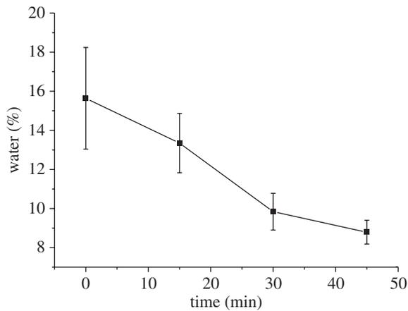
Figure 2. Water content in samples varies with different exposure time to the vacuum conditions of the SEM instrument. The water content was measured as weight lost during the TGA tests when heating the samples up to 200°C.
