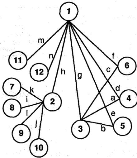
Figure 4: Component-fastener relationship graph for the assembly shown in Figure 1.
