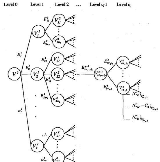
Figure 8: recycling cost in the disassembly tree
