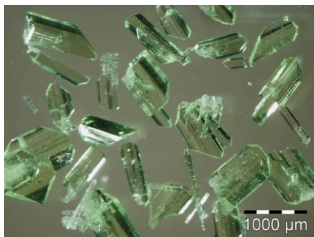
Figure 24. Crystals of \text{PrPO}_4 grown by chemical vapor transport.
