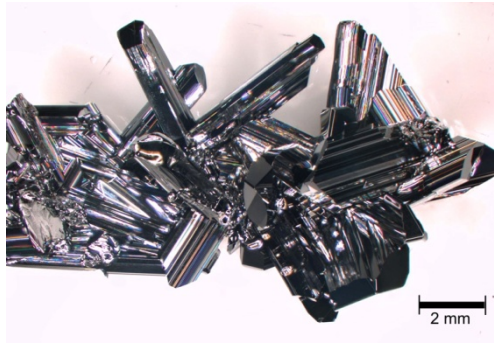
Figure 30. Crystal of ZrAs_2 grown by chemical vapor transport.
