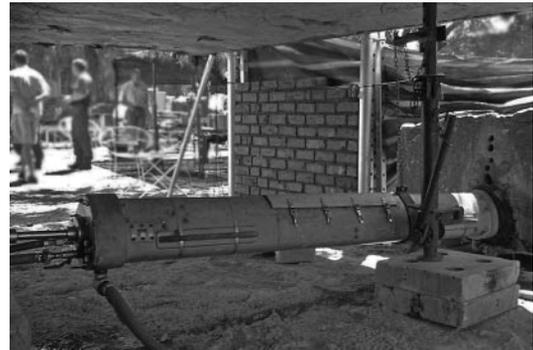
Fig. 1. Self-propelled drill in the above-ground artificial stope.
