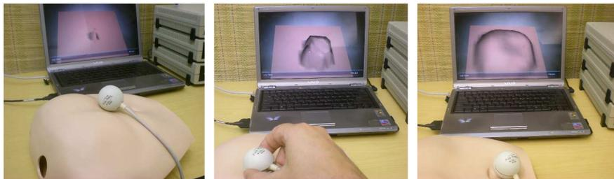
**Fig. 12** Scanning SimMan abdomen module: sensor alignment (left), scanning in progress (middle), completed mesh (right) Grid size 40x40 cm, 20x20 points. Scanning time: under 2 minutes.
