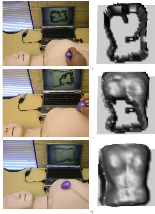
**Fig. 13** Scanning Anne Torso: initial contour (top), intermediate shape (middle), and final mesh (bottom). The 3D mesh snapshots are shown as produced by the scanner, without retouching (see also Fig. 15). Grid size 40x40 cm, 40x40 points. Scanning time: about 8 minutes.
