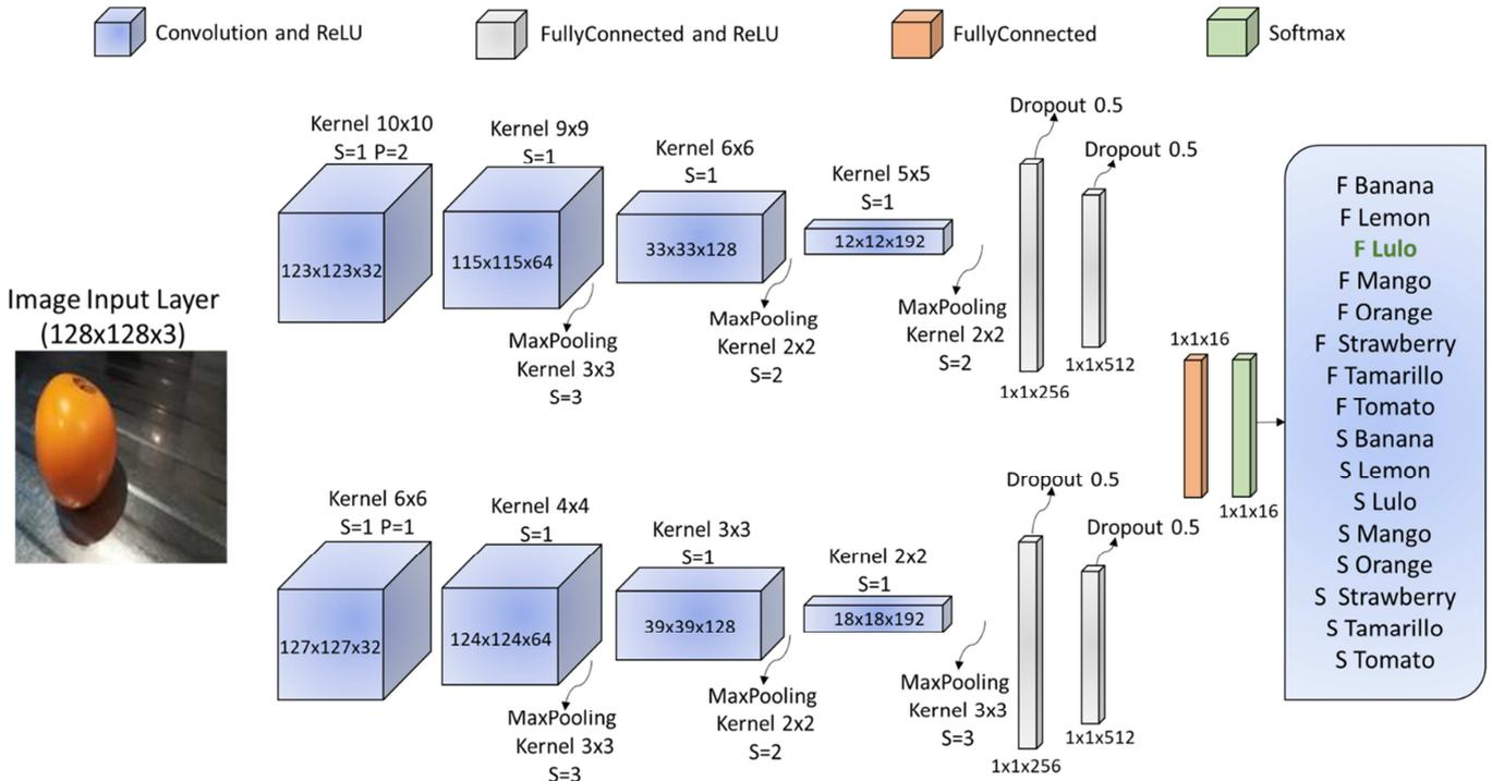
Fig. 3 Architecture of the DAG-CNN where S refers to the Stride and P to the Padding.
