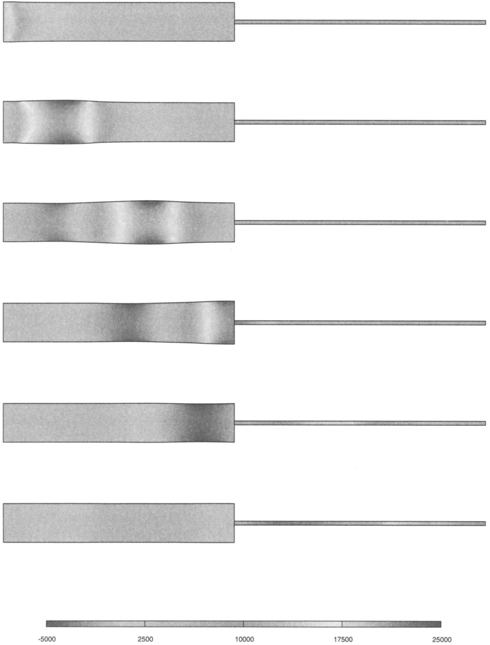
FIG. 11. Coupling 2D simulation with the 1D reduced model; pressure distribution every 5 ms, starting from t = 1 ms.
