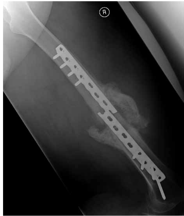
Figure 6 — Fatigue failure of LCP fixed on a fractured femur of 47-year-old male after 6 months of bearing partial weight.
